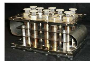
Prototype of hydrogen release unit for dehydrogenation of LOHC.
